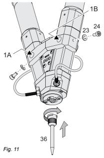
**Tip:** Connecting a hose to the mixing pipe can protect the eco-DUO450 from being wetted with the material.
