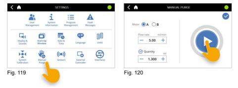
The purge quantity and the flow rate can be individually set for each component. Manual purging is started by pressing the START/STOP-button.
