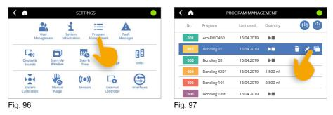
In the program manager you can edit, duplicate and delete the individual programs. You can also save all installed programs simultaneously to a USB stick (Fig. 97). This makes it possible to create a backup copy.
