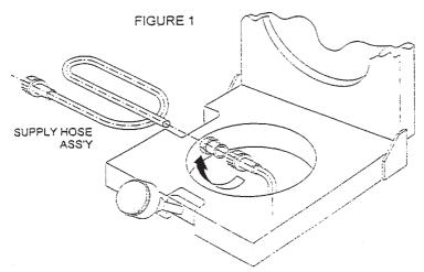
7. Close Lid, swing Knob Assembly (7) up to vertical position and hand tighten Knob firmly.
