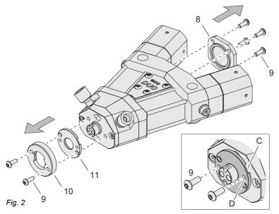
Tip: If the eccentric ring (11) cannot be easily removed (stuck with material), then
