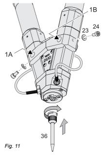
**Tip:** Connecting a hose to the mixing pipe can protect the eco-DUO330 from being wetted with the material.
