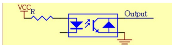
FIG. 24: Example of I/O output port driving
