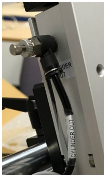
FIG. 8: Z-Axis Drive Cylinder Setup
